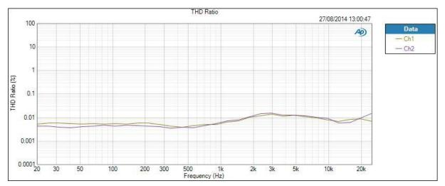
Figure 5 - THD vs. Frequency shows the THD+N of the Cyrus class D amplifier is consistent with frequency and does not shoot up at higher frequencies like many other class D amplifiers. This is due to the optimised PCB layout; feedback and reconstruction filter design along with the low error rate of the second order sigma delta modulator. (9)
