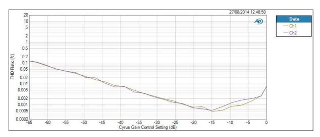
Figure 3 - THD vs. Gain Control Setting on Cyrus Preamplifier with -6dBFS Input
