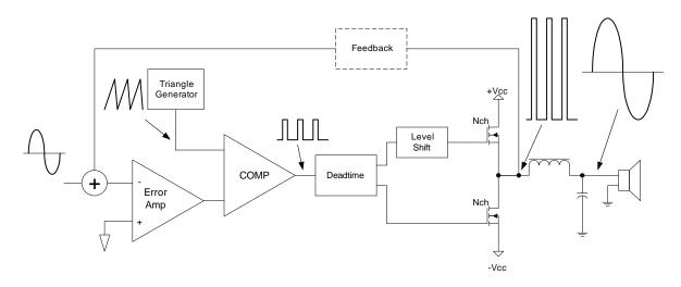
Figure 1 – Simplified Class D amplifier
